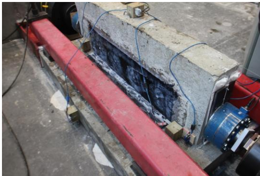
Strengthened specimen in the experimental setup
