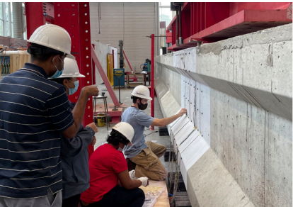
Above: The Marc Basnight Bridge was built to replace the Herbert C. Bonner Bridge in 2019. Photo courtesy of HDR. Left: Dr. Giorgio Proestos' research group marking cracks during the testing of a Bonner Bridge Girder at the Constructed Facilities Lab.
