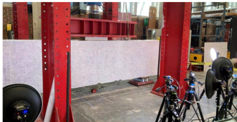
1) Large-scale deep beam experiments conducted using DIC
