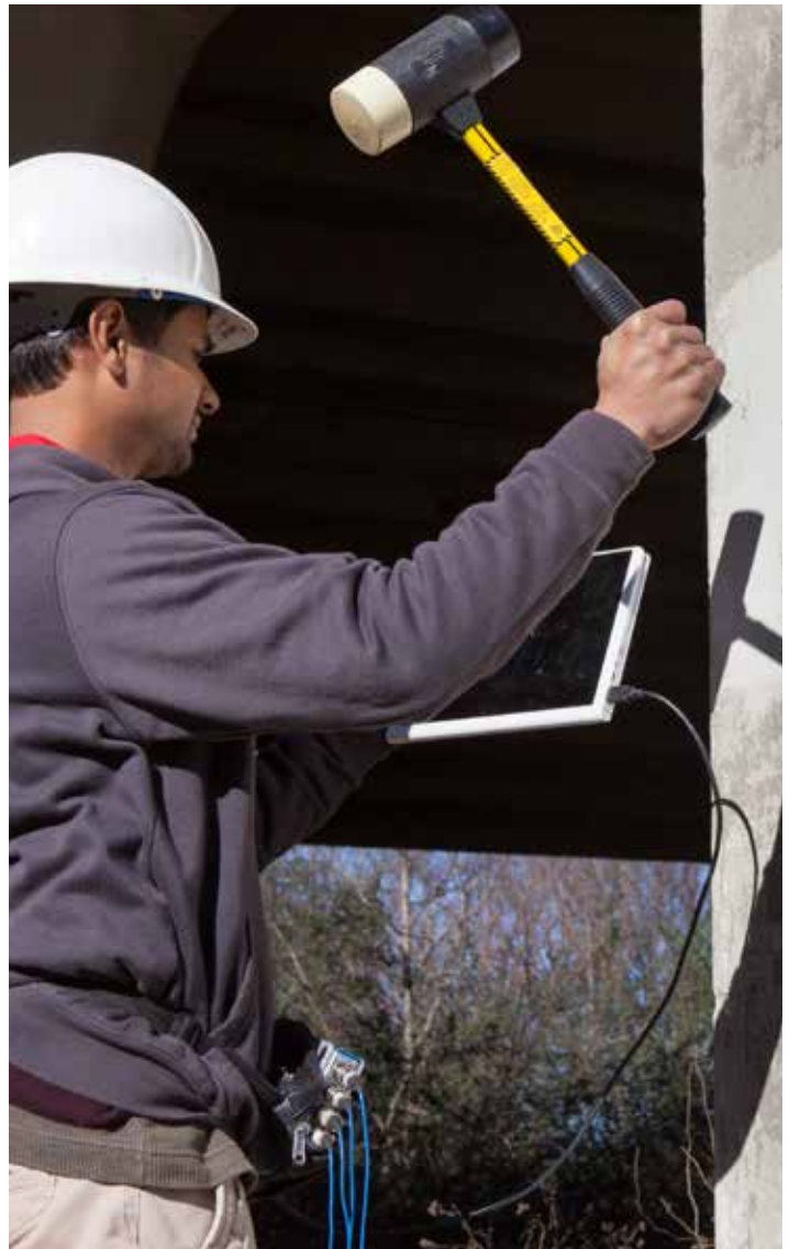
Vivek Samu (Ph.D. 2018, MSCE 2014) field testing Effective Dispersion Analysis of Reflections (EDAR) equipment in 2015. Samu continues his work as a postdoctoral researcher with Dr. Guddati.
