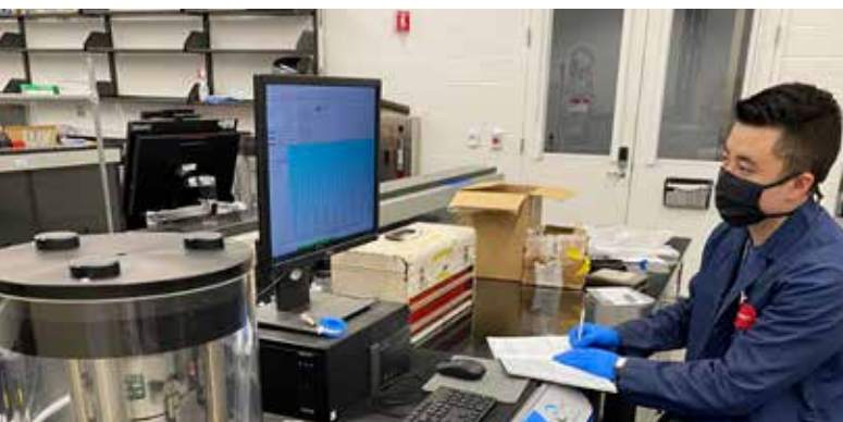
In the asphalt multiscale testing lab, Ph.D. student Kazuo Kuchiishi calibrates the load cell of the Asphalt Mixture Performance Tester (AMPT). This instrument is used to measure the stiffness, cracking resistance and deformation resistance of asphalt mixtures. Kuchiishi is conducting research to improve the test method used to measure the dynamic modulus of asphalt mixtures.
