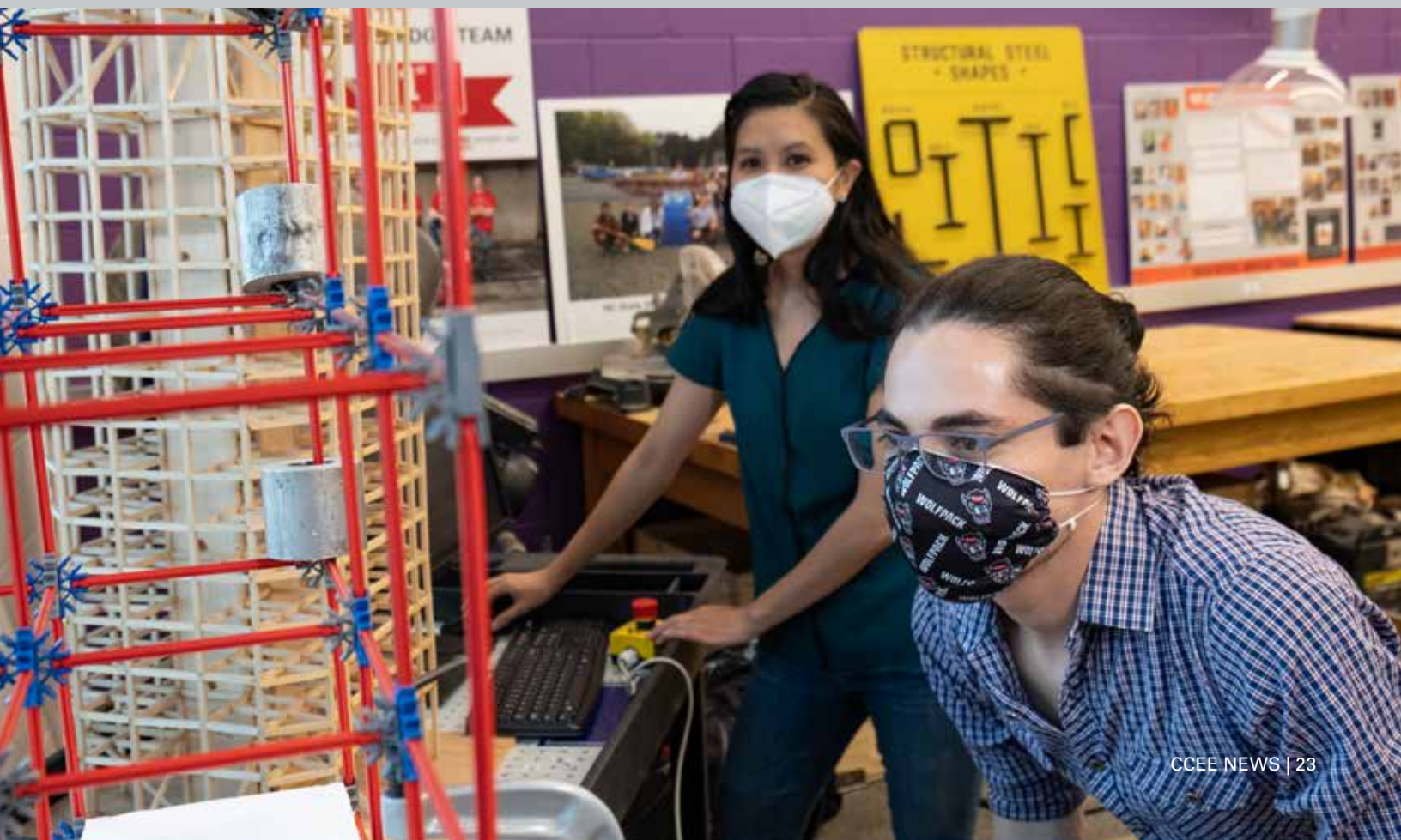
Below, Ph.D. students Jessi Thangitham and Julio Samayoa are demonstrating structural response using a shake table. They are shaking a structure made from K'NEXs to explore the behavior under earthquake loading.
