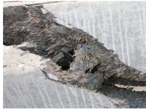
UHPC Ledge Punching Shear Failure: Left, overall view; right, close-up showing fibers
