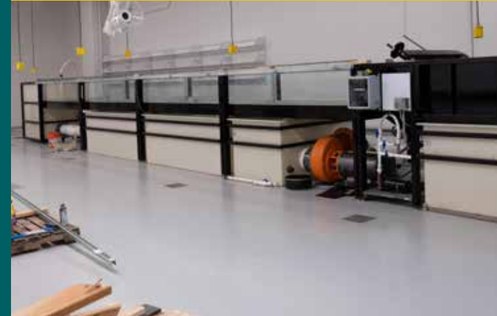
Above: Pieces of a sediment recirculation flume built in and shipped from Minnesota are unloaded. Below: Once assembled in the Hydraulics Lab the flume will be 45 feet long by 3 feet wide and will be capable of 6 cubic feet per second of water flow.
