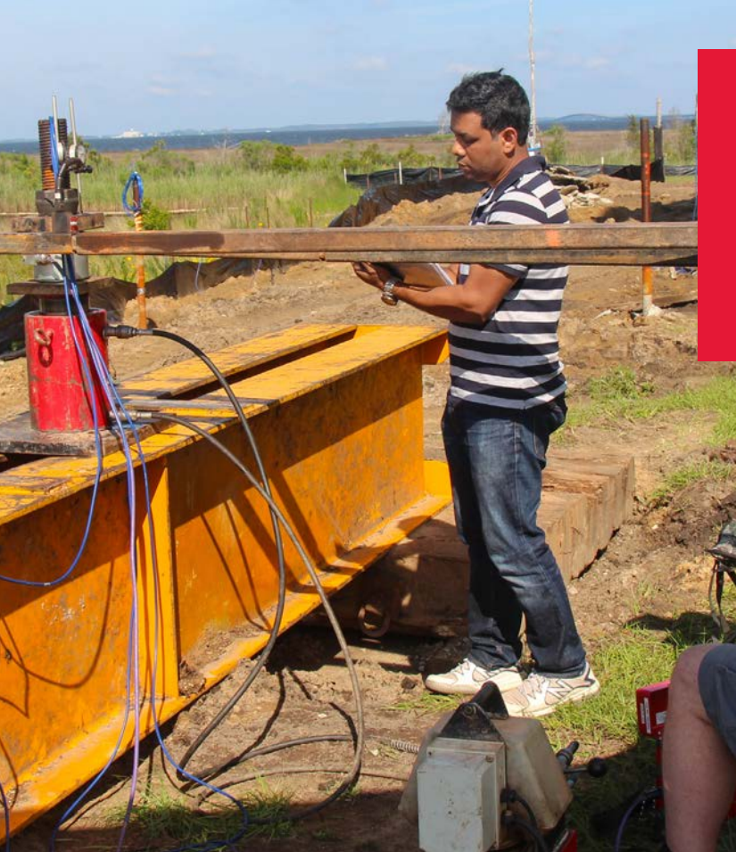
Ph.D. student Mohammed Ahsanuzzaman records the displacement of the top of the micropile at different loading conditions, as well as the strains at different depths of the micropile.
