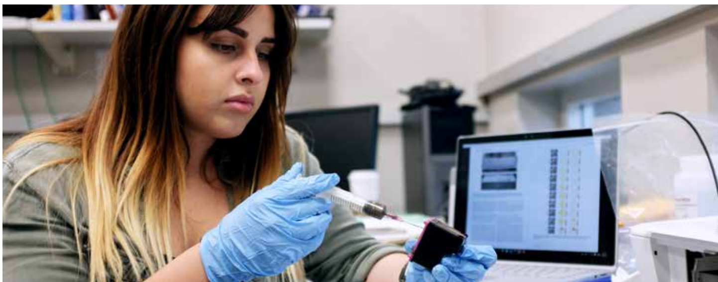
Paola Armada Rodriguez helped develop a technique using inkjet printers with modified cartridges to print sensors used in electrical impedance tomography. Armada worked closely with Professor Mohammad Pour-Ghaz, and Ph.D. students Danny Smyl and Reza Rashetnia.
