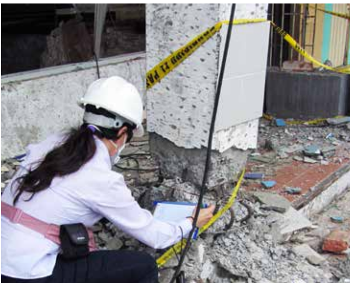
Gabby Haro documents damaged reinforcement at the base of a column.
