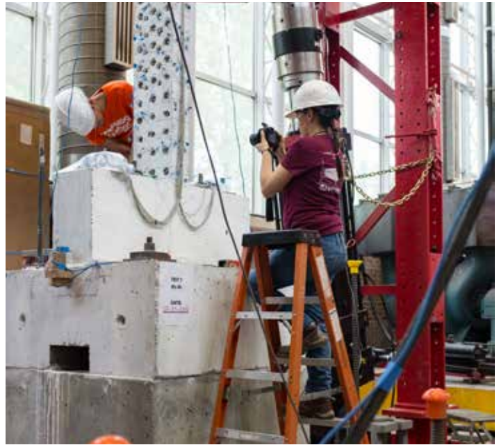
Gabby Haro carefully documents cracks in a wall pier test conducted for the Alaska Department of Transportation.
