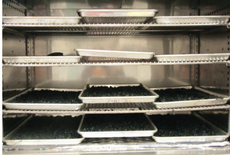
Loose mix asphalt undergoing long-term aging in an oven.
