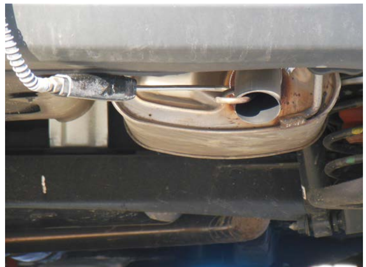
Sampling of tailpipe exhaust from a passenger car.
