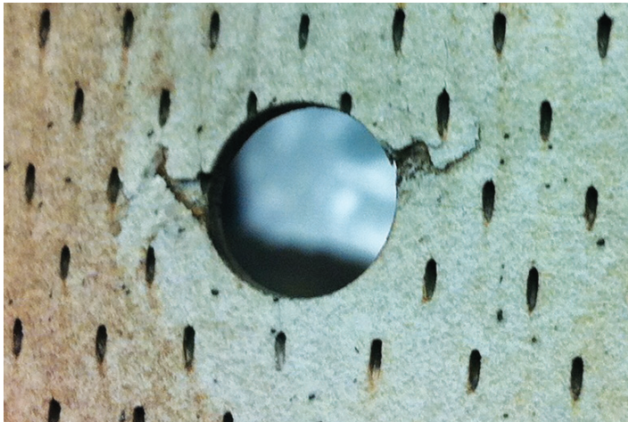
Top: Jet engine gas turbine (Courtesy of Honeywell Aerospace). Bottom: Close up of a gas turbine combustor liner with a premature crack.
