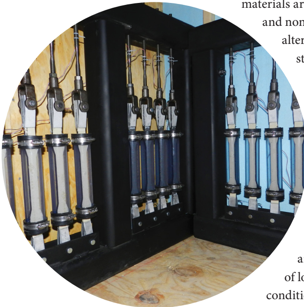
Fiber reinforced polymer (FRP) specimens under sustained loading and simultaneous exposure to moisture and aggressive agents for accelerated aging.
