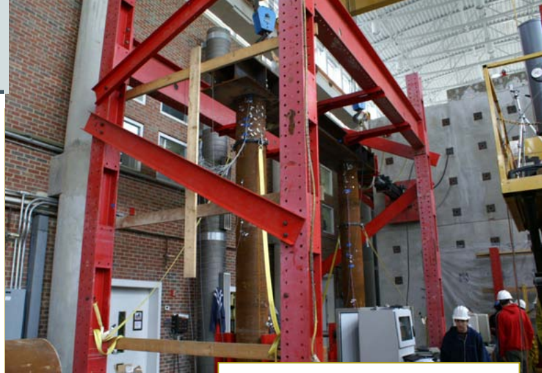
Seismic testing of a typical Alaska bridge at the Constructed Facilities Laboratory.
