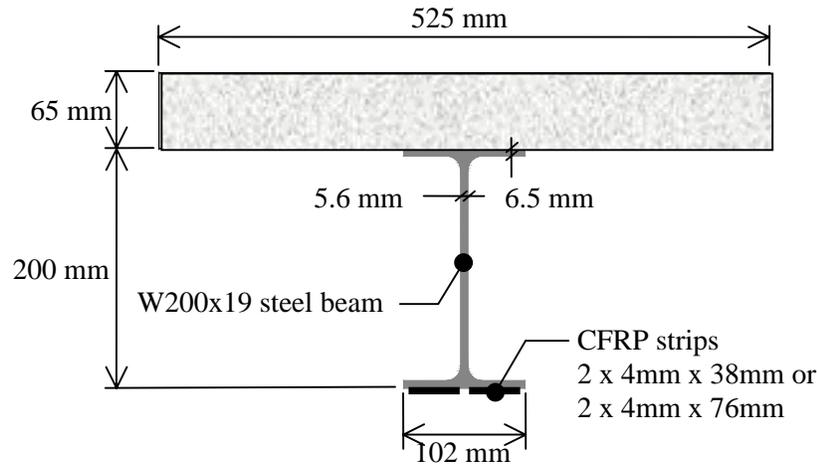
**Figure 1: Cross-section of a typical test beam**
