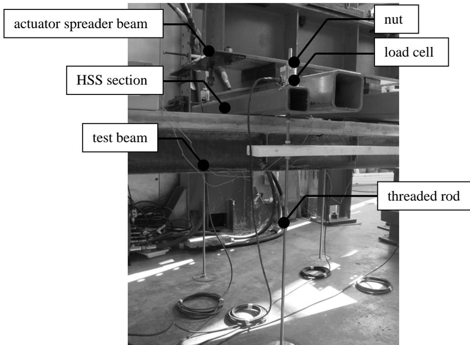
*Figure 3: Independent dead-load apparatus*
