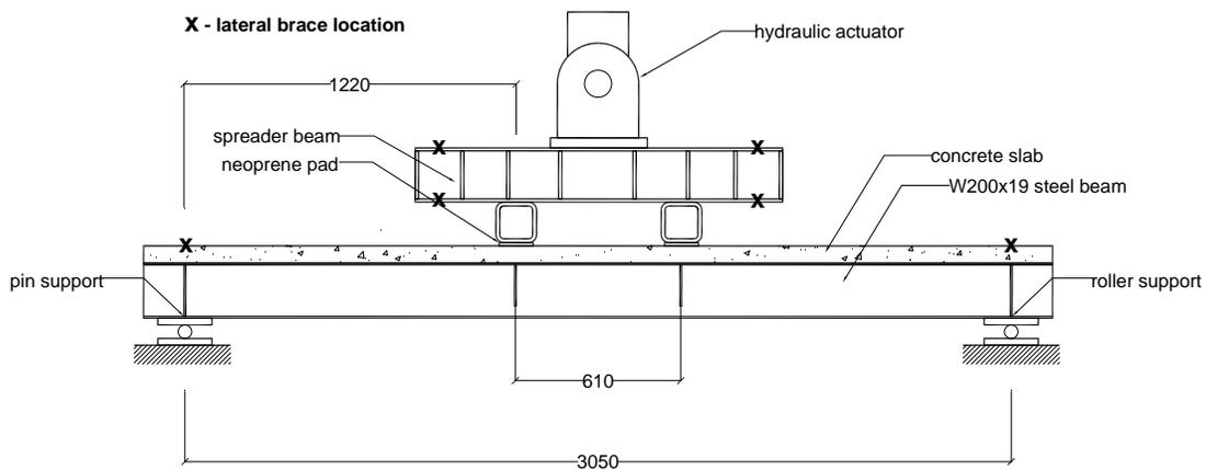
**Figure 2: Beam test setup**
