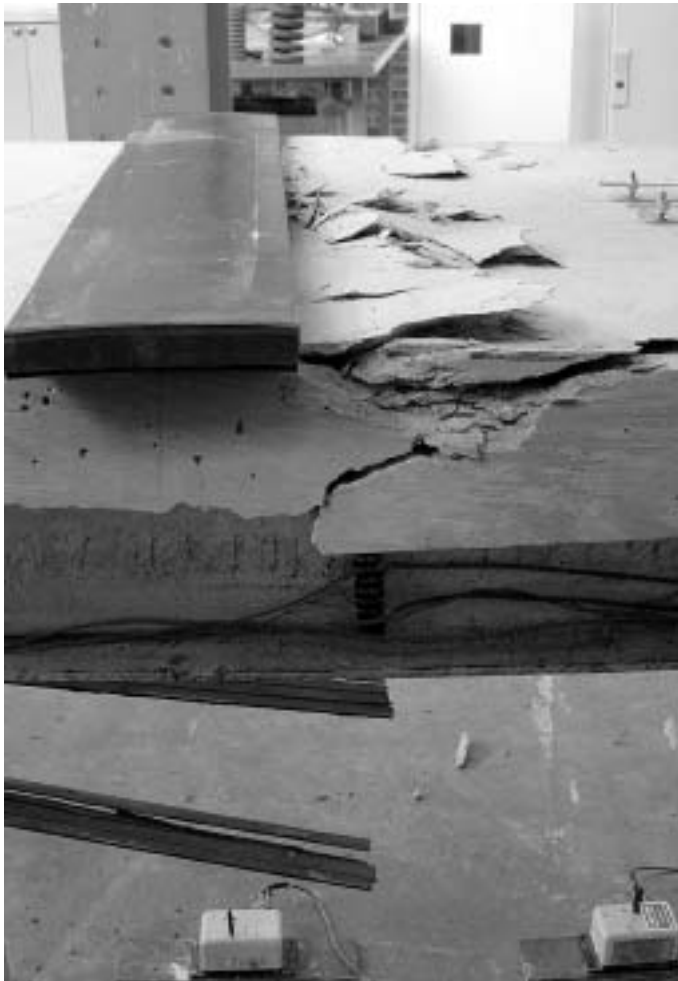
Figure 13. Concrete crushing failure and CFRP strip rupture of steel-concrete composite girder (CGAB-I).
