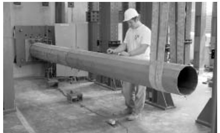
Figure 4. Test setup for scaled monopoles.
