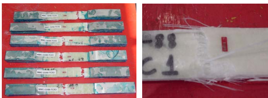
Fig. 9 Failure mode for the tensile specimens
