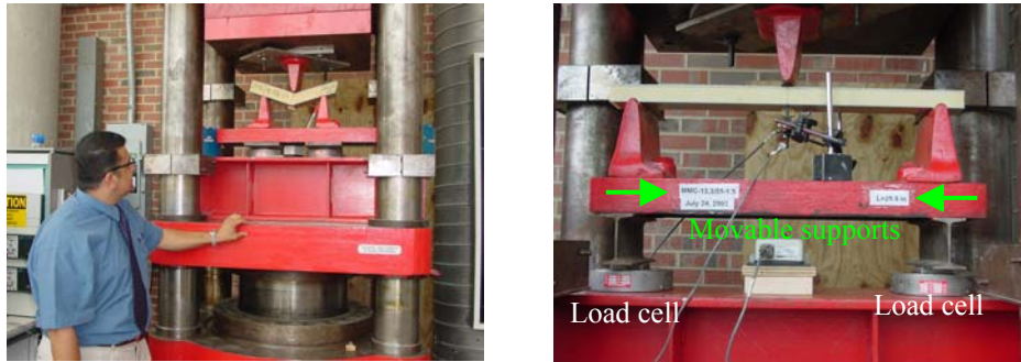
Fig. 10 Flexural test setup using a single concentrated load
