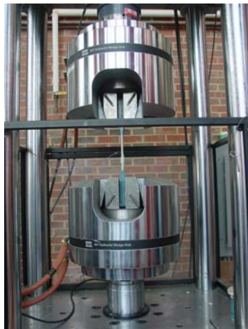
Fig. 8 Test set-up for the tension specimens
