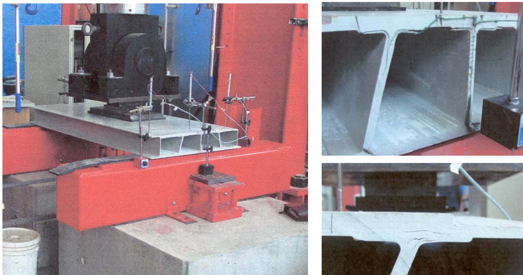
Fig. 1 Typical delamination of the web from face sheets for pultruded modular FRP bridge decks [Nelson and Rizkalla, 2003]
