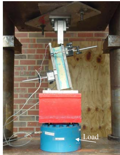
Fig. 5b Test setup for the shear tests
