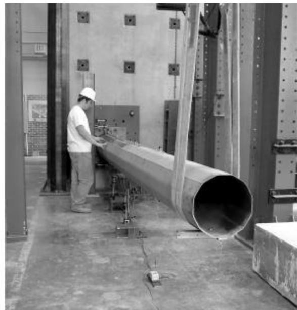
Figures 7a & b. Test setup for scaled steel monopoles
