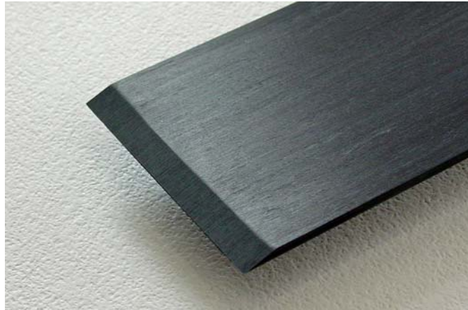
Figure 3. Configuration of taper at end of strip
