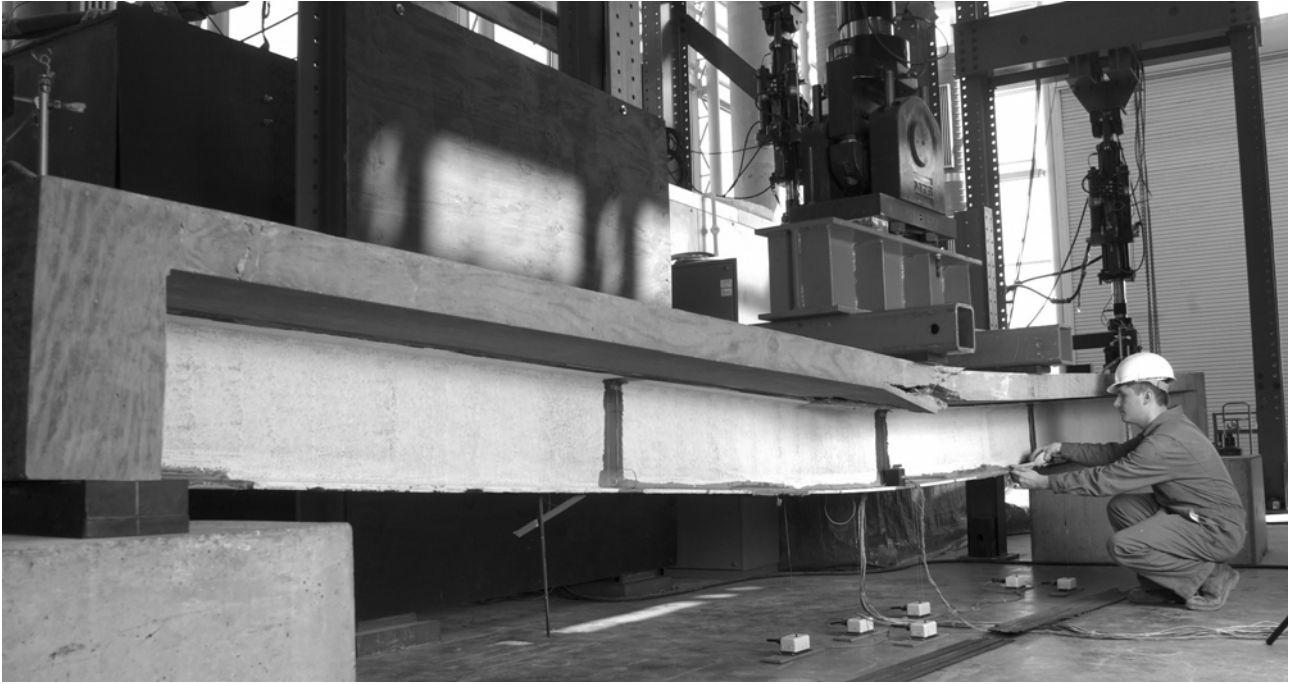
Figure 3 Steel-concrete composite beam HM-7.6-AB after failure
