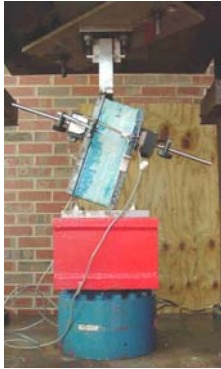
Figure 6 – Instrumentation and test set-up for shear tests
