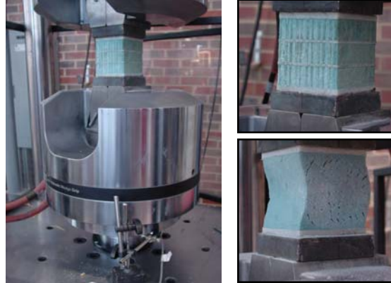
Figure 7 – Test set-up for the compression specimens
