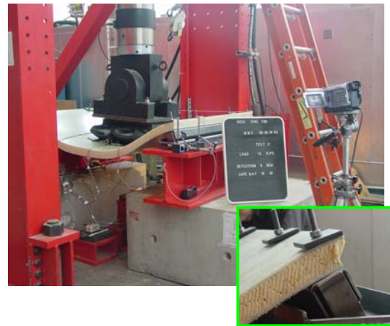
Figure 5 – Failure mode of panel 2
