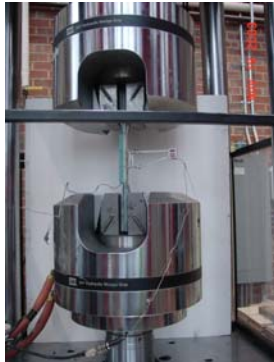
Figure 8 – Test set-up for the tension specimens
