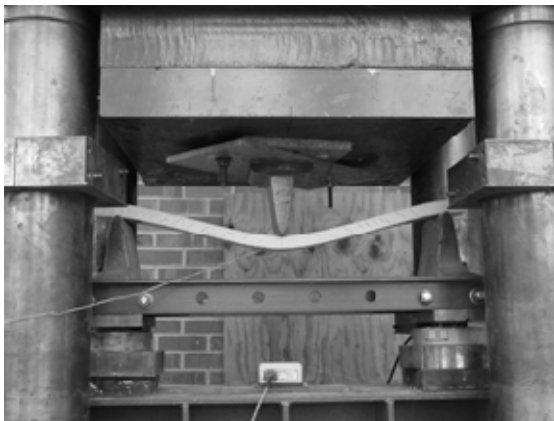
Figure – 14 Test set-up for flexural test
