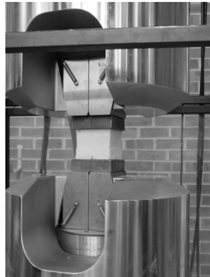
Figure – 16 Test set-up for compression specimens
