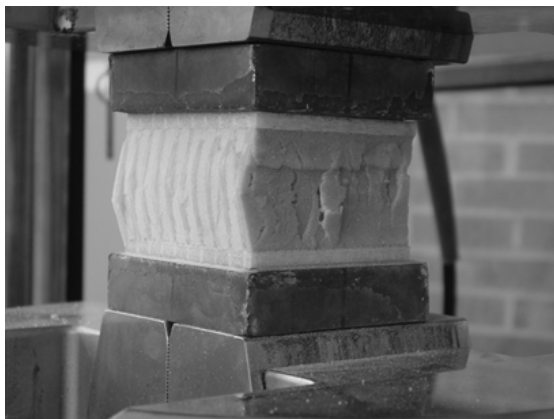
Figure – 21 Buckling of through thickness fibers at failure
