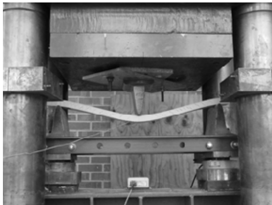
Figure – 14 Test set-up for flexural test
