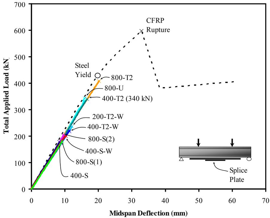
**Figure 9:** Measured load-deflection relationship for the tested beams
