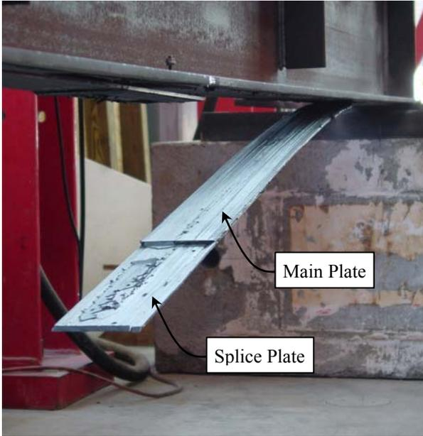
**Figure 8:** Typical debonding failure of a splice beam
