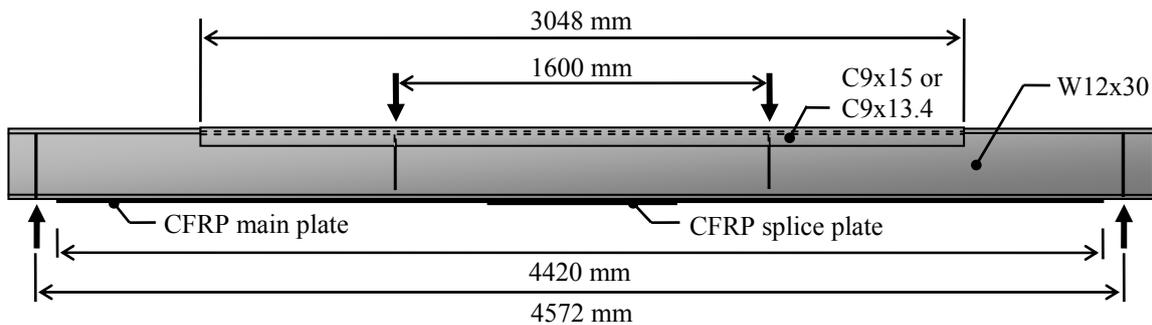
**Figure 3:** Schematic of test beam and test setup
