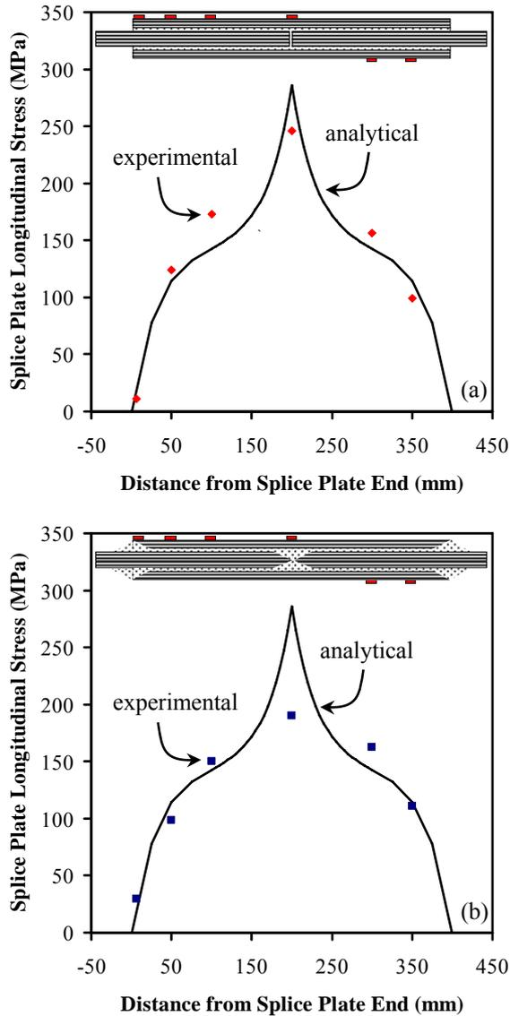
**Figure 6:** Longitudinal stress distribution in the splice plate for coupon (a) 400-S and (b) 400-T2(1)
