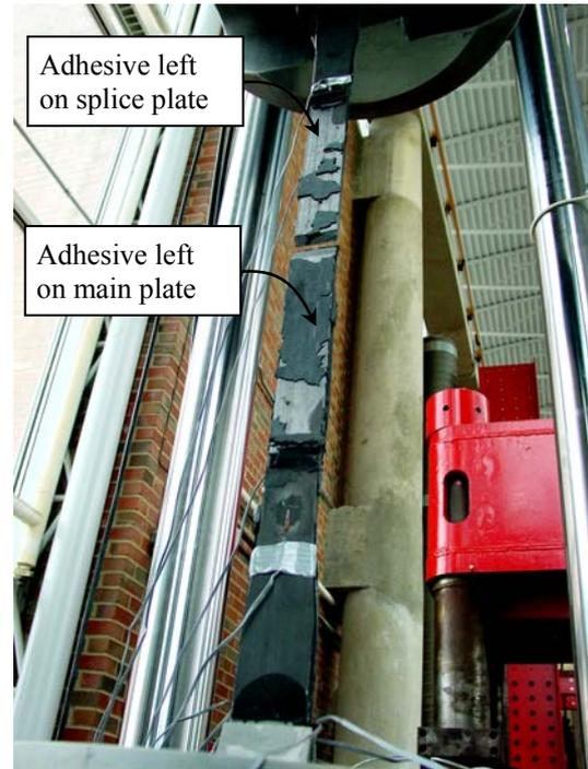
**Figure 5:** Typical failure of splice coupon
