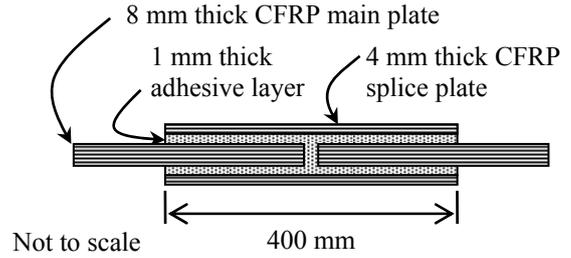
**Figure 1:** Typical double-lap shear coupon
