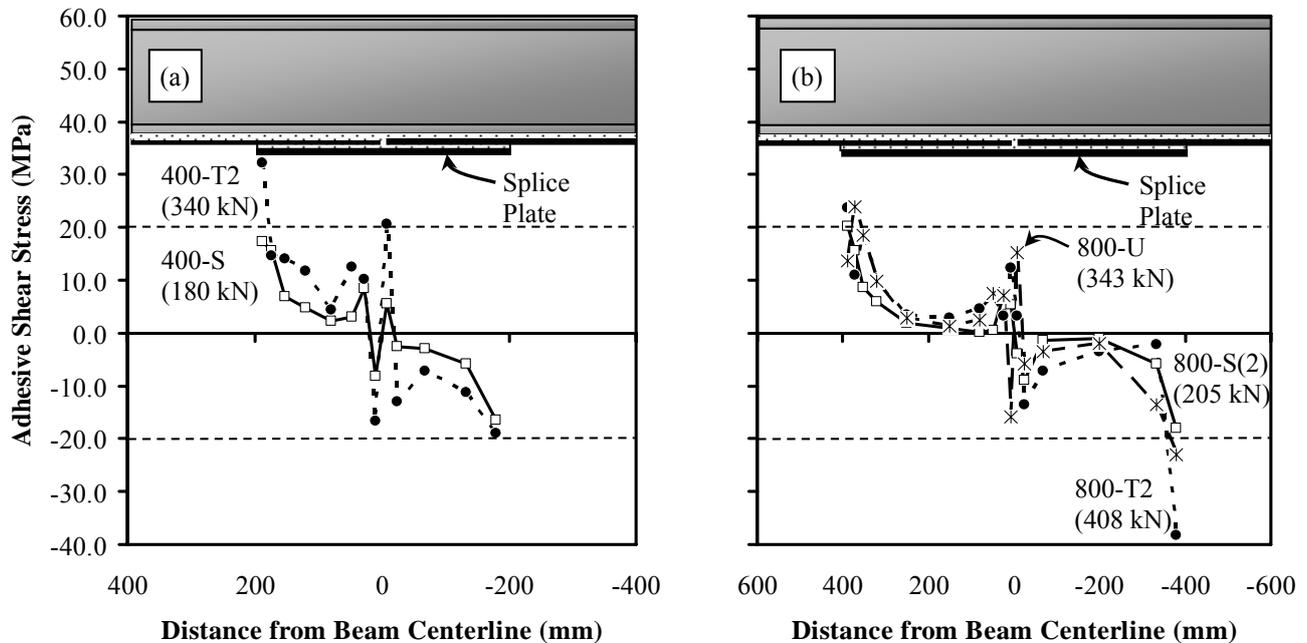
**Figure 11:** Experimentally obtained adhesive shear stress distributions for the tested beams with (a) 400 mm long splice plate (b) 800 mm long splice plates at failure
