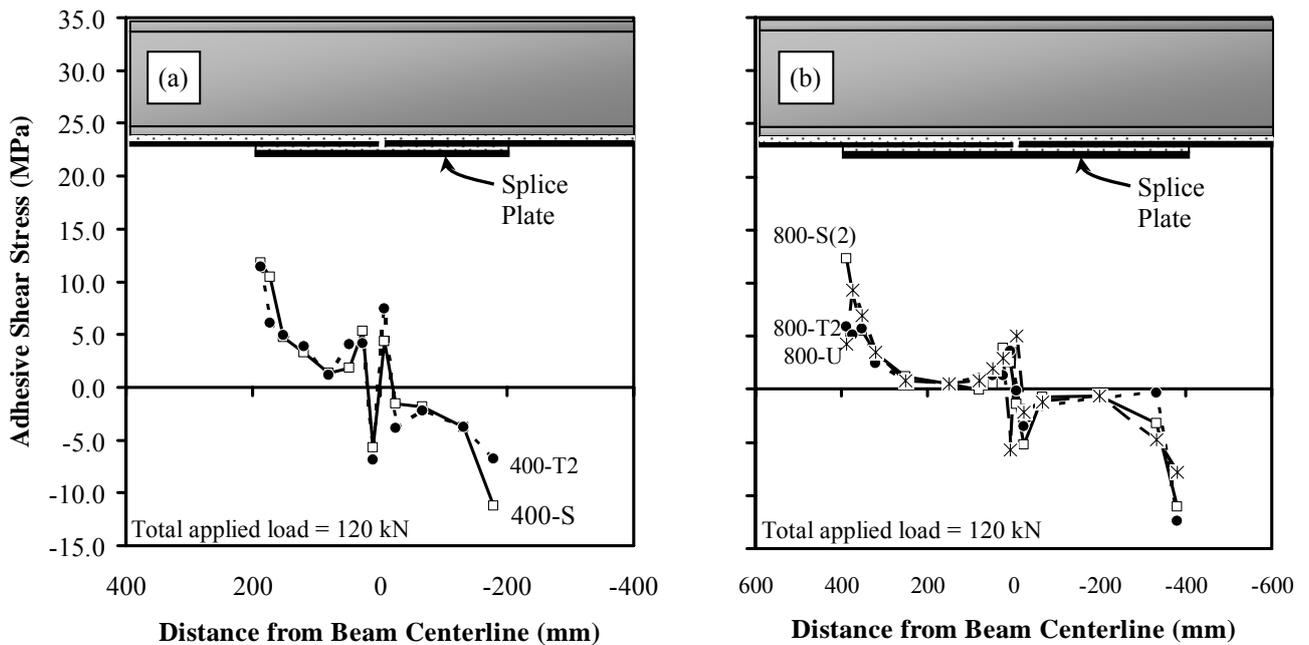
**Figure 10:** Experimentally obtained adhesive shear stress distributions for the tested beams with (a) 400 mm long splice plate (b) 800 mm long splice plates at a load level of 120 kN
