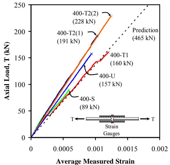
**Figure 7:** Load-strain behavior at centerline of splice
