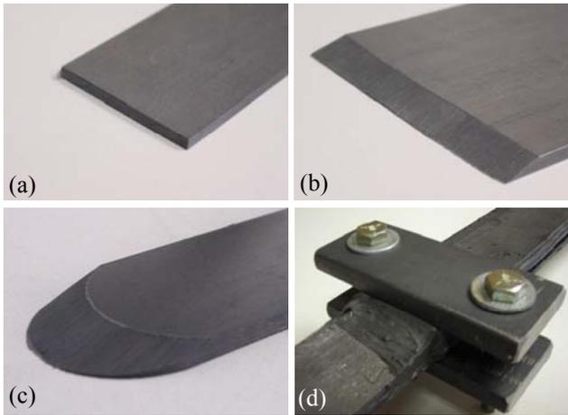
**Figure 2:** (a) square, (b) tapered, (c) rounded and (d) clamped plate ends
